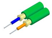
Fiber indoor cable, 1.6 mm diameter, Plenum rated, Zipcord 2-fiber, Singlemode G.657.A2/B2, Feet jacket marking, Green jacket color
