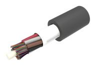
Fiber Indoor/outdoor Cable, Low Smoke Zero Halogen / 24 fiber Microsheath, Tube Colours as per DIN/VDE 0888, Gel-free, Singlemode G.657.Al, Meters jacket marking, Black jacket color, Dca flame rating
