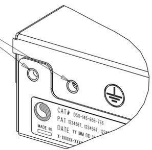
DETAIL GROUNDING VIEW SCALE 1.000 (SECURE)
