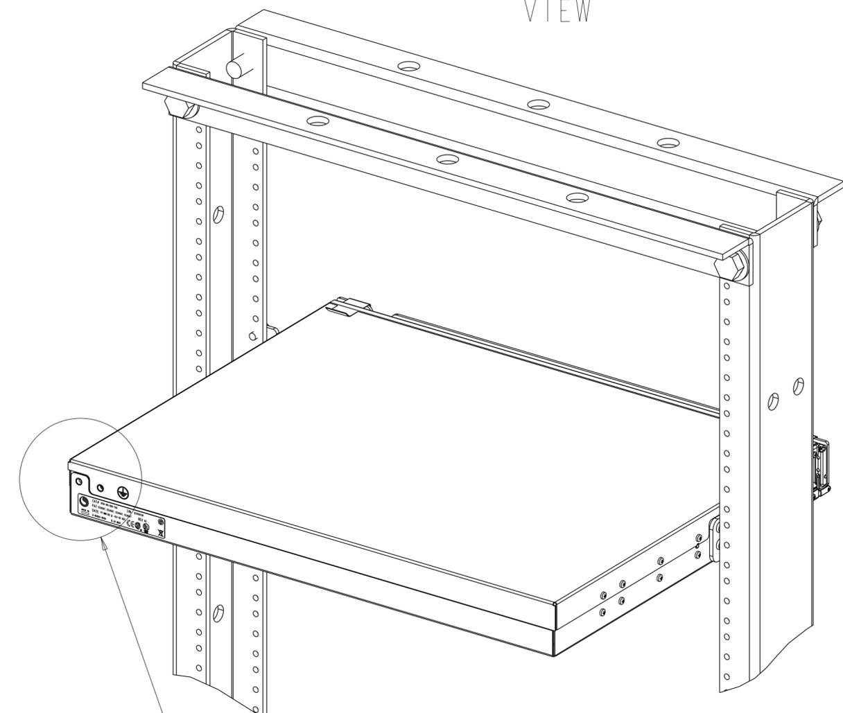
INSTALL EHD PANEL TO FRAME USING (4) SCREWS AND (4) STAR WASHERS PROVIDED WITH UNIT.
