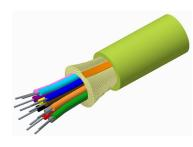
Fiber indoor cable, Low Smoke Zero Halogen Distribution, 24 fiber singleunit, Multimode OM5, Meters jacket marking, Lime green jacket color
