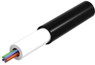
Fiber OSP cable, LightScope® ZWP Blown Single Jacket All-Dielectric Outdoor Central Tube Construction 6 fiber, Singlemode G.657.A2, Gel-filled, Meters jacket marking, Black jacket color
