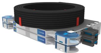
FACT® Fiber Optic Pre-cabled Chassis, gray, 2E high, 96-port, singlemode, loaded with LC/UPC Duplex adapters and C-grade pigtails, SMOUV splice tray type, 10m in/outdoor Microsheath cable, G657A1, EN50575 CPR Cable EuroClass Dca, right-hand patch
