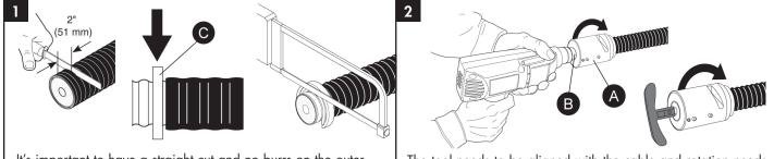
It's important to have a straight cut and no burrs on the outer conductor. Rotate saw guide halfway through the cut to ensure saw is always resting on the guide and last saw stroke should be soft to avoid tearing the outer conductor.
