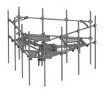
PIM Optimized Adjustable Monopole Platform with 15ft Face - 2-7/8in OD Face Pipes & Top Rail - Includes (12) 2-7/8in OD x 96in Antenna Pipes
