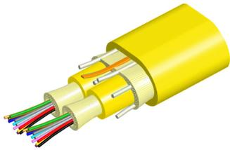
Fiber indoor cable, Low Smoke Zero Halogen Riser MPO Trunk, 16 fiber with 8 fiber 2.0 mm subunits, Singlemode G.657.A2/B2, Feet jacket marking, Yellow jacket color, Dca flame rating
