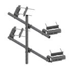
Tower Face Mount with dual 8 ft x 4-1/2 in OD face pipe supports and (2) 2-3/8 in x 63 in Strut supports, includes pipe
