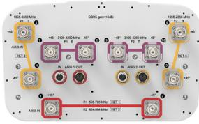
10-port sector antenna, 2x 698-894, 4x 1695-2360 and 4x 3100-4200 MHz, 65° HPBW, 3x RETs and 2x SBTs
