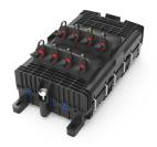
Mini-OTE 300-Series, Optical Terminal Enclosure, 8-port prodigy connector, with integrated 1x8 splitter, black, with grounding, external mounting. Splitter outputs connected to terminal housing ports, maximum 26 splices.
