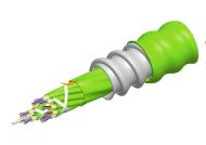
Fiber indoor cable, LazrSPEED® Plenum MPO Trunk, interlocking aluminum armored with plenum jacket, 72 fiber multi-unit with 8 fiber subunits, Multimode OM5, Feet jacket marking, Lime green jacket color
