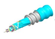
Fiber indoor cable, LazrSPEED® Riser/LSZH rated, MPO Trunk, interlocking aluminum armored, Multimode OM4, 48 fiber, Gel-free, Feet jacket marking, Aqua jacket color, B2ca flame rating
