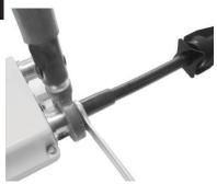
Torque the connection using the approprite tools.
