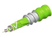
Fiber indoor cable, Plenum MPO Trunk, interlocking aluminum armored with plenum jacket, 96 fiber multi-unit with 16 fiber subunits, Gel-free, OM5 multi-mode, Feet jacket marking, Lime green jacket color
