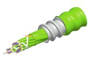
Fiber indoor cable, Plenum MPO Trunk, interlocking aluminum armored with plenum jacket, 64 fiber multi-unit with 16 fiber subunits, Gel-free, OM5 multi-mode, Feet jacket marking, Lime green jacket color
