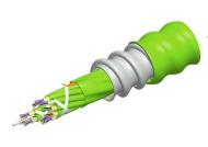
Fiber indoor cable, Plenum MPO Trunk, interlocking aluminum armored with plenum jacket, 48 fiber multi-unit with 16 fiber subunits, Gel-free, OM5 multi-mode, Feet jacket marking, Lime green jacket color
