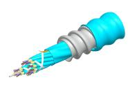
Fiber indoor cable, Plenum MPO Trunk, interlocking aluminum armored with plenum jacket, 192 fiber multi-unit with 16 fiber subunits, Gel-free, OM4 multi-mode, Feet jacket marking, Aqua jacket color
