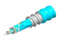
Fiber indoor cable, Plenum MPO Trunk, interlocking aluminum armored with plenum jacket, 64 fiber multi-unit with 16 fiber subunits, Gel-free, OM4 multi-mode, Feet jacket marking, Aqua jacket color
