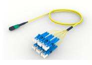
Ultra Low Loss (ULL) Singlemode MPO12 (Unpinned) to LC/UPC, Fiber Extension Cable Assembly, 12-Fiber, Low Smoke Zero Halogen, Method-A Polarity: Method A
