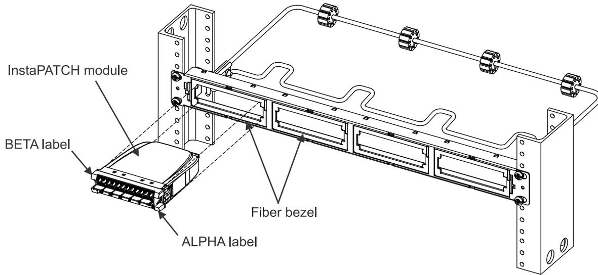
1. Orient module in ALPHA or BETA position as required and insert into one of the openings in the panel.
