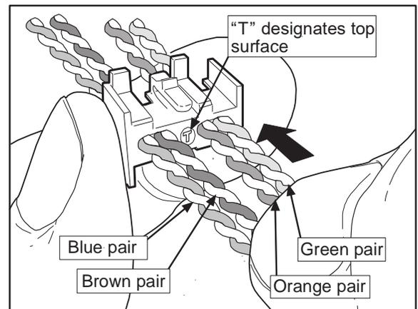
Figure 2. Feed Pairs into Termination Manager
