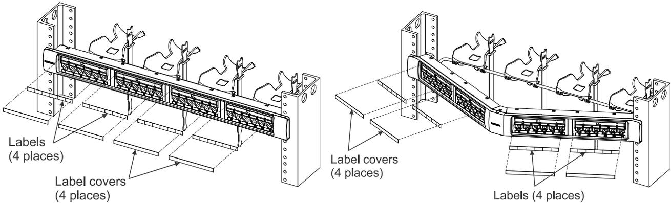
1. Print the port designations on the white label cards provided. Slide labels and label covers into the label holders from either end. Each label holder will accommodate labels up to .265 inches (6.7mm) high x 3.50 inches (89mm) wide.
