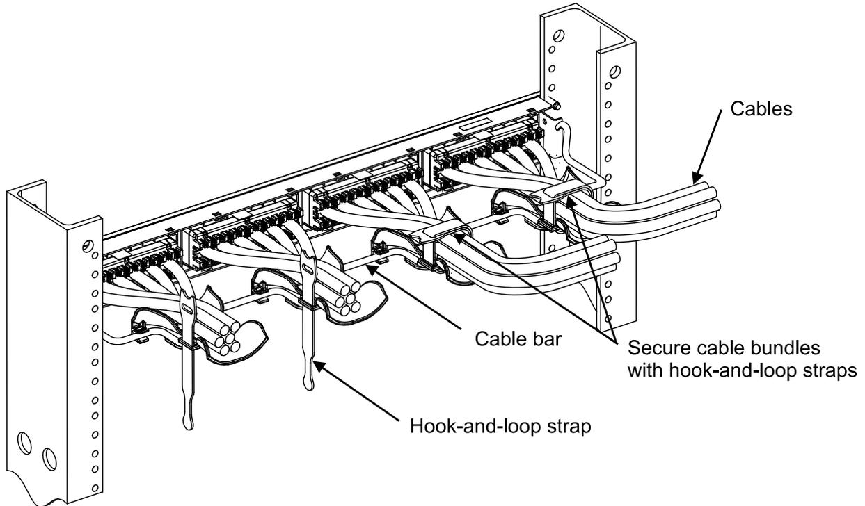
2. Attach cable bar to rear of panel. For 48-port panels, two cable bars are provided.
