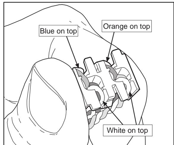
Figure 3. Fold Pairs Back into Slots
