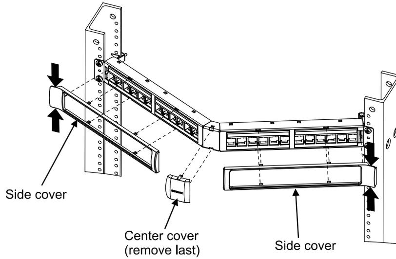
1. When removing either the flat or angled panel side cover(s), grip cover on the top and bottom at the outside edge where shown by arrows and pull forward. As cover tabs release, position fingers close to tabs to apply further pulling force.
