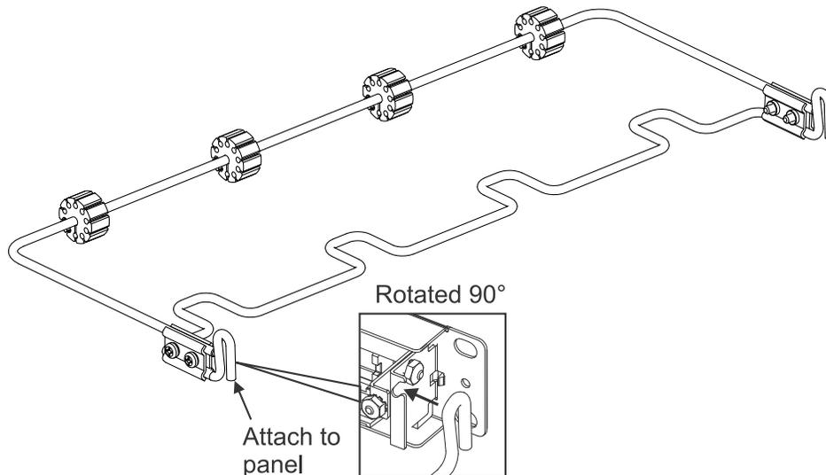
1. Attach fiber management bar to rear of panel immediately behind the fiber row. Place hook at both ends of bar into slots in panel brackets as shown.
