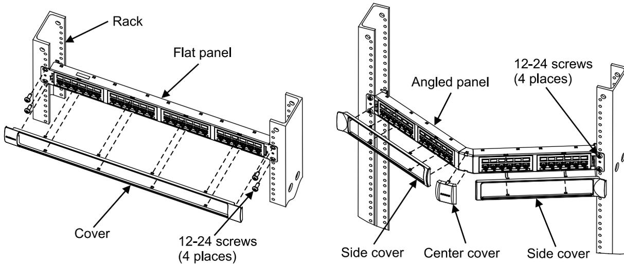
1. Mount panel to rack using the four 12-24 mounting screws provided. After securing panel to rack, snap the Evolve cover(s) onto the front of the panel.
