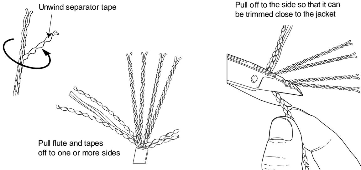
Preparation of the **SYSTIMAX GigaSPEED X10D 91B series cable, 95B series cordage, or Xpress 88 series cable** is shown above. For complete instructions on preparing these cables for termination, see instruction sheet 860469402.
