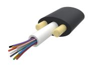
Fiber outdoor drop cable, LightScope® ZWP Self-Supporting All-Dielectric, Singlemode G.652.D and G.657.Al, 12 fiber Arid Core construction, Gel-filled, central loose tube, Feet jacket marking, Black jacket color, 5000 ft
