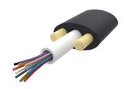
Fiber outdoor drop cable, LightScope® ZWP Self-Supporting All-Dielectric, Singlemode G.652.D and G.657.Al, 4 fiber Arid Core construction, Gel-filled, central loose tube, Feet jacket marking, Black jacket color, 5000 ft
