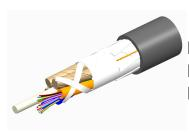
Fiber indoor/outdoor cable, LazrSPEED®, Single Jacket All-Dielectric, Plenum Rated, , 12 fiber multimode OM5, Gel-Free, Stranded Loose Tube, PVDF jacket, Black jacket color, Feet cable marking
