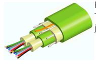
Fiber indoor cable, LazrSPEED® Low Smoke Zero Halogen Riser MPO Trunk, 48 fiber with 24-fiber, 3.0 mm subunits, Multimode OM5, Feet jacket marking, Aqua jacket color, B2ca flame rating
