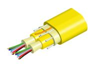
Fiber indoor cable, Low Smoke Zero Halogen Riser MPO Trunk, 48 fiber with 24-fiber, 3.0 mm subunits, Singlemode G.657.A2/B2, Feet jacket marking, Yellow jacket color, B2ca flame rating
