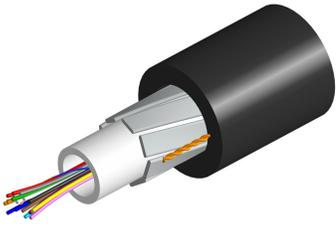
Fiber indoor/outdoor cable, Gel-filled Central Tube, 12 fiber, Singlemode G. 652.D and G.657.A1, Meters jacket marking, Black jacket color
