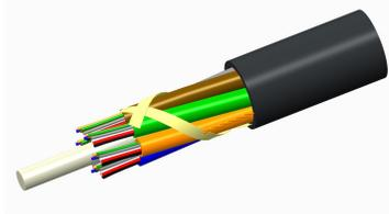
Fiber OSP cable, LightScope® ZWP Blown Micro Single Jacket All-Dielectric Outdoor Stranded Loose Tube Arid-Core™ Construction, 144 fiber, Singlemode G.657.A2, Gel-filled, Meters jacket marking, Black jacket color
