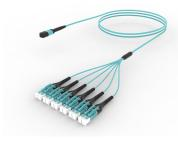
Ultra Low Loss (ULL) OM4 MPO12 (Pinned) to LC Uniboot, Fiber Array Cable Assembly, 12-Fiber, Dual Rated (OFNR/LSZH)
