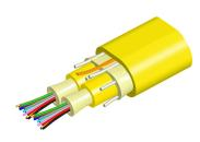
Fiber indoor cable, Low Smoke Zero Halogen Riser MPO Trunk, 16 fiber with 8 fiber 2.0 mm subunits, Singlemode G.657.A2/B2, Feet jacket marking, Yellow jacket color, B2ca flame rating
