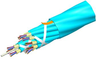
Fiber indoor cable, LazrSPEED® Low Smoke Zero Halogen Riser MPO Trunk, 48 fibers, with 2.0mm Subunits, 48 fiber, Multimode OM4, Gel-free, Feet jacket marking, Aqua jacket color, B2ca flame rating
