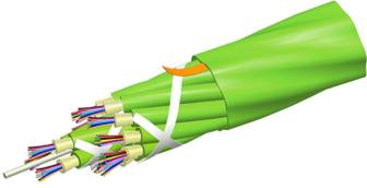
Fiber indoor cable, LazrSPEED® Low Smoke Zero Halogen Riser MPO Trunk with 2.0mm Subunits, 24 fiber, Multimode OM5, Gel-free, Meters jacket marking, Lime green jacket color, B2ca Flame rating
