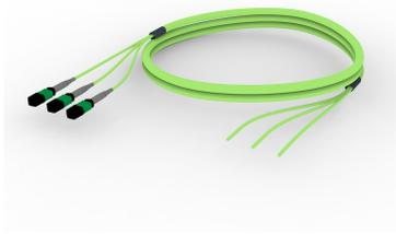
Ultra Low Loss (ULL) OM5 MPO8 APC (Non-Pinned) to Unconnectorized, Fiber Trunk Cable Assembly, 24-Fiber, LSZH B2ca
