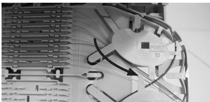
9.5.7. To store over-length around the islands, start the routing following the arrow (which is also indicated on the tray).
