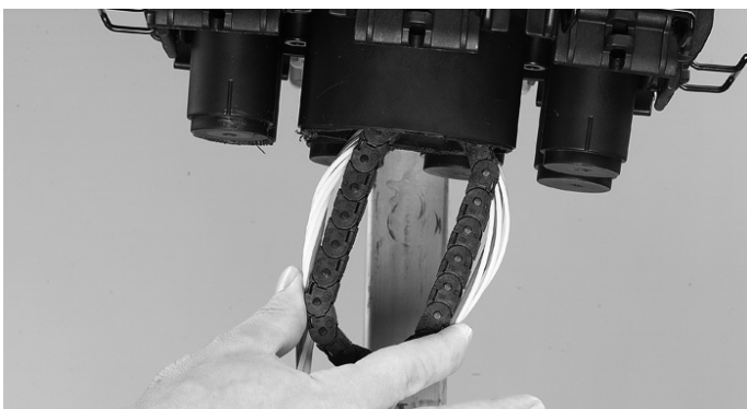
7.2.5.3. Push the loose tubes through the oval port. The LCIT can be used to avoid kinking of the loose tubes.
