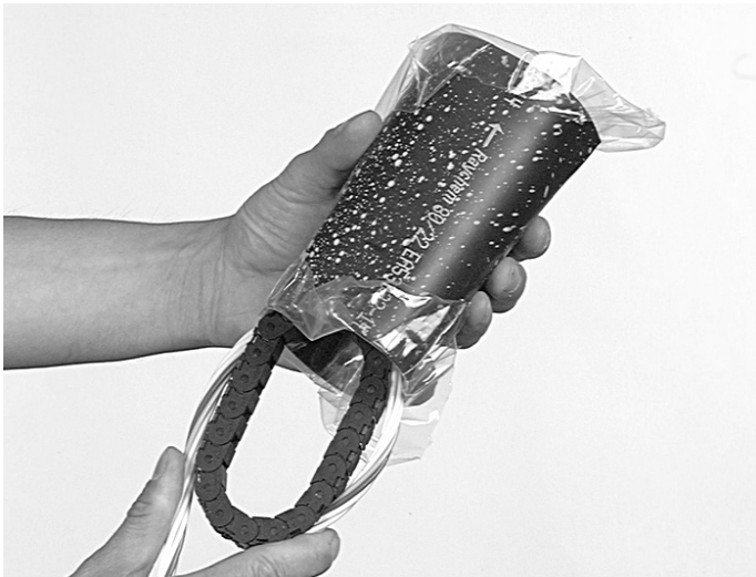
7.2.5.2. If sealing with heatshrink: Push the loose tubes through the oval sleeve. The non-coated edge of the sleeve (arrow) should be pointed towards the base of the closure. Make sure the hotmelt in the sleeve is protected against dirt. The plastic bag of the packaging can be used to protect it.
