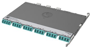
Propel ULL Multimode OM4 MPO-08 Distribution Module, 12 duplex LC to 3X8f MPO/UPC non-pinned, Method B Enhanced
