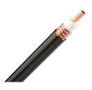
AVA5-50, HELIAX<sup>®</sup> Andrew Virtual Air<sup>™</sup> Coaxial Cable, corrugated copper, 7/8 in, black PE jacket (Halogen free jacketing non-fire-retardant) tested C-Band and CBRS qualified.
