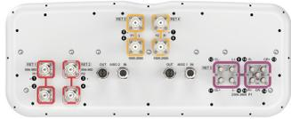
16-port sector antenna, 4 x 694-960 MHz (R1-R2), and 4 x 1695-2690 MHz (Y1-Y2) 65° HPBW, 8 x 2300-3800 MHz (P1), 90° HPBW, 5 x RET
