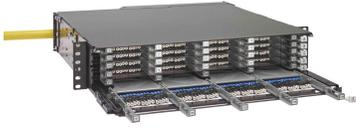
EHD-2U Pre-stubbed Patch Panel with LC/UPC Adapter and 288f I/O, Riser/LSZH rollable ribbon cable, right cable entry, singlemode with cable length in meters from 25m to 400m in 25m increments
