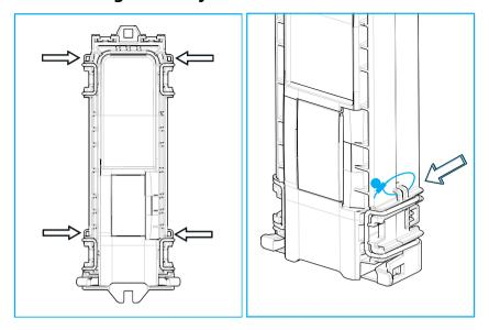
1 There are 4 locations to secure the closure with a securuty wire. Push the wire through the holes on the top and bottom cover and seal the wire per local practice.
