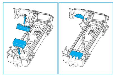
1 Install the Octopus<sup>™</sup> gel block with the plastic support of the gel block down. Push on the gel block until it is secured by the attachment points on the housing.
