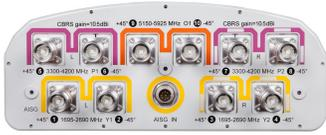
10-port small cell antenna, 4x 1695–2690, 4x 3300–4200 and 2x 5150–5925 MHz. 65° HPBW, Internal RET and SBT
