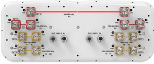
14-port sector antenna, 2x 694-862 (R1), 2x 880-960 (R2), 2x 694-960 (R3), 8x 1695-2690 (Y1/Y2/Y3/Y4) MHz, 65° HPBW, 7x RET.
