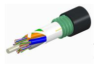
Fiber indoor/outdoor cable, TeraSPEED®, Single Jacket/Single Armor, Low Smoke Zero Halogen (LSZH), Singlemode G.652.D and G.657.A1, 36 fiber, Gel-Free, Stranded Loose Tube, Meters jacket marking, Black jacket color, Cca flame rating
