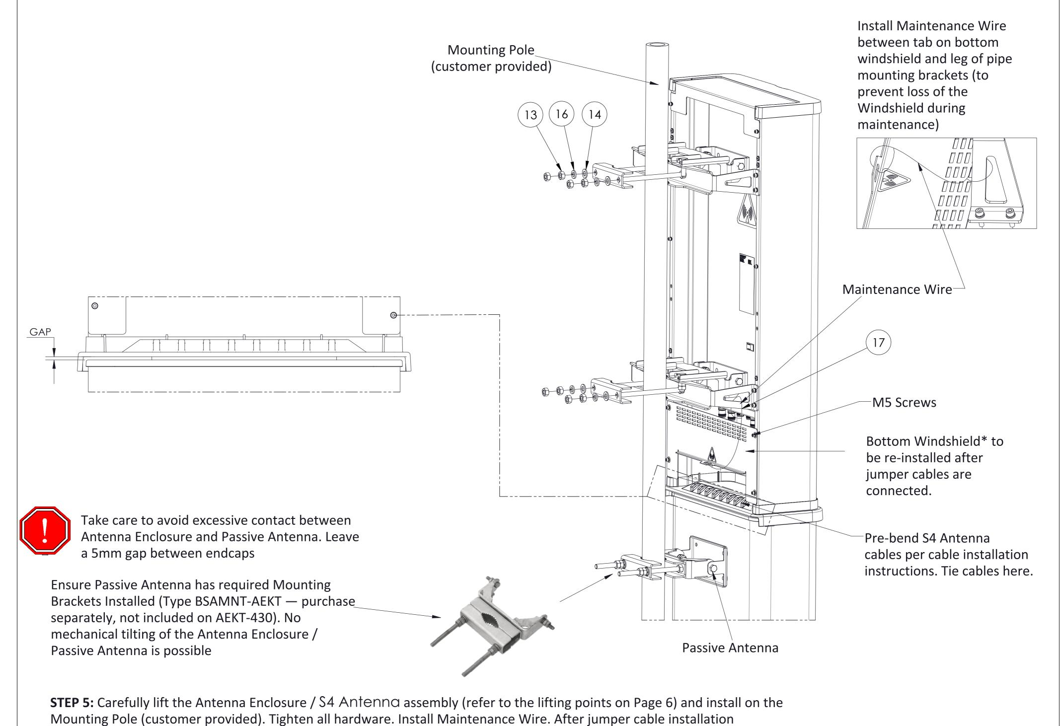
re-install Bottom Windshield\*. NOTE: The Passive Antenna should be installed first before installing the Enclosure.
