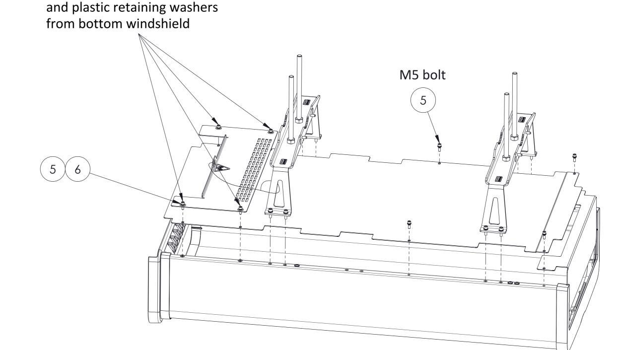
**STEP 2:** CAREFULLY place the empty Enclosure front face down on a clean, flat surface taking steps to protect the unit (use a suitable cushioning material). Remove all 3 Windshields and both Pipe Mounting Brackets (if fitted) and retain all hardware.
