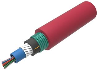
Fiber Indoor/Outdoor cable, TeraSPEED®, 120 min Fire Survival, Low Smoke Zero Halogen (LSZH), 12 fiber, Gel-Filled, Central Loose Tube, Singlemode G.652.D and G.657.A1, Meters jacket marking, Black jacket color
