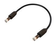
HELIAX® 1/2" SureFlex® Jumper with interface types 4.3-10 Male and 7-16 DIN Male with HELIAX® SureGuard weatherproofing, 10 m
