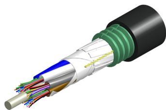
Fiber indoor/outdoor cable, TeraSPEED®, Single Jacket/Single Armor, 90 min Fire Survival, Low Smoke Zero Halogen (LSZH), 72 fiber, Singlemode G.652.D and G.657.A1, Gel-Filled, Stranded Loose Tube, Black jacket color, Meters cable marking
