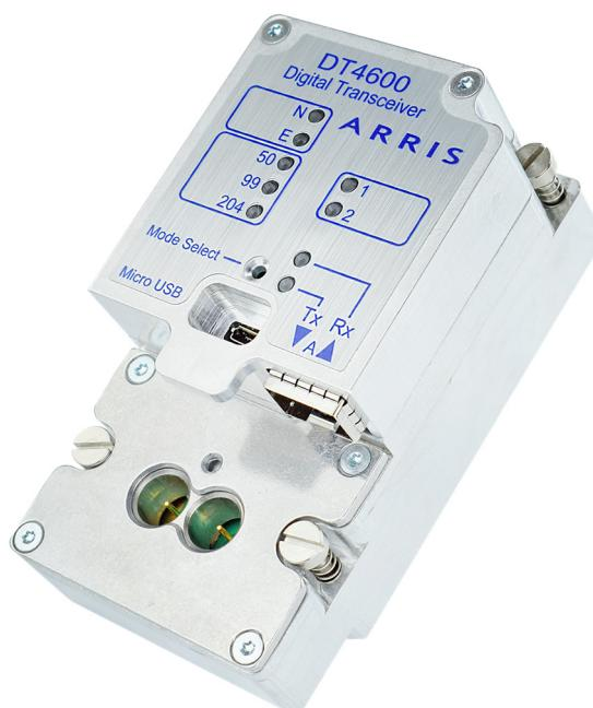
The DT4600N features user selectable operating modes of 5–204 MHz or 5–100 MHz (covering 5–65, 5–85 MHz etc.) RF return bandwidths. Either range can be operated as a single channel “1-fer” or a two channel “2-fer” return path. For 5–204 MHz range, a Headend CH3000 chassis based DR3600N Return Receiver is required. For the 5–100 MHz range, a DR3600N or DR3450N Return Receiver can be used. The DT4600N (100 MHz mode) also supports RF Returns to CHP Chassis based CHP-D2RRX-85-AA-S Receivers.
