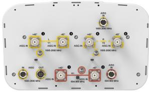
6-port sector antenna, 2x 694–960 and 4x 1695–2690 MHz, 65° HPBW, 3x RET with manual override and internal Bias-Tee's.
