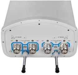
4-port multibeam antenna, 4x 1710–2180 MHz, 2x 38° HPBW, RET compatible
